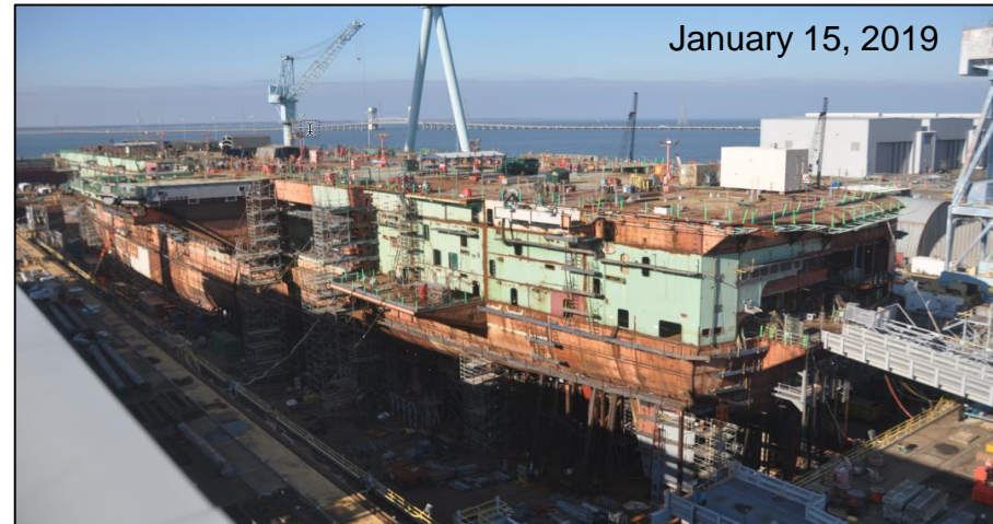
Hull Erect is nearing completion, moving into Hull Blast & Coat
